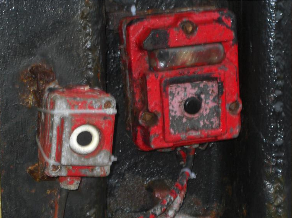
MV MSC Hina: damaged fire dampers, defective manual call points for fire alarm, damaged emergency stop for mooring winch
